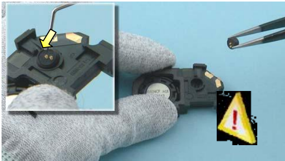
15) Use the dental tool to lever out the microphone. Be careful not to damage yourself or the microphone!
