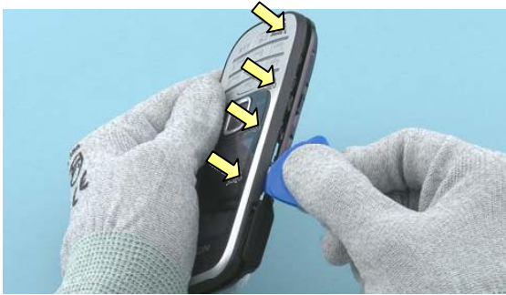
7) Continue to release the snaps on the left side of the A-COVER with the SRT-6.
