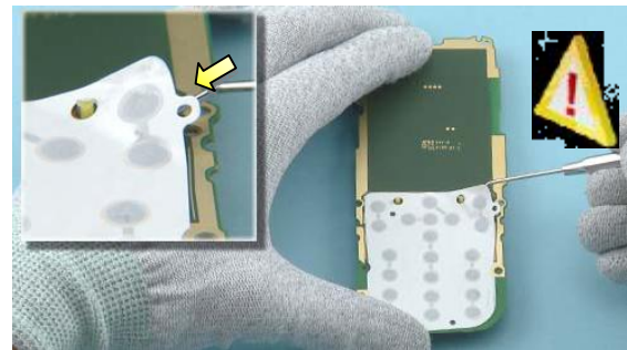
24) Use the dental tool to lift an edge of the DOME SHEET. Be careful not to damage the DOME SHEET or the PWB!
