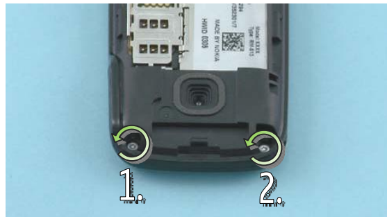
6) After the A-COVER is in place, tighten the two Torx+ 4 screws to the torque of 14 Ncm in the order shown.
