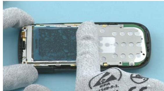
10) Protect the LCD with a protective film.
