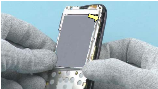
3) Place the ENGINE MODULE in its place with respect to the snap on the D-COVER.
